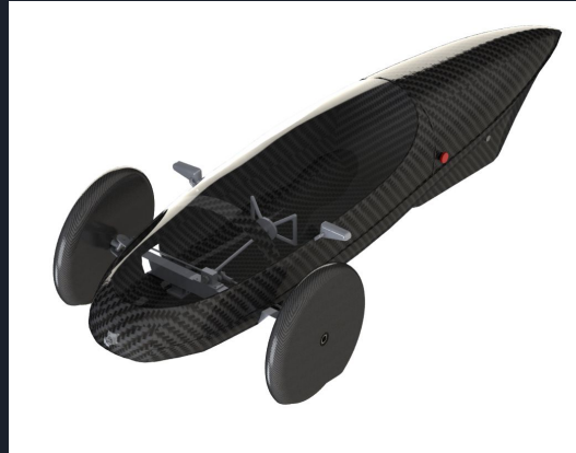
New design. Vehicle has a carbon fiber body and aluminium steering rack
